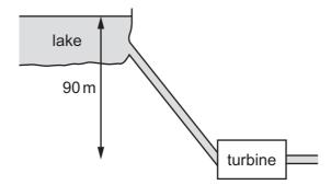
The mass flow rate of the water is  $2400 \text{ kg min}^{-1}$ . The turbine has an efficiency of 75%.
