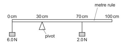
The rule balances when a weight of 6.0 N is hanging from the zero mark and a weight of 2.0 N is hanging from the 70 cm mark.
