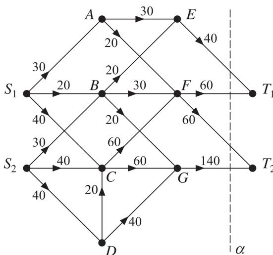
The diagram represents a system of pipes through which fluid can flow from two sources,  $S_1$  and  $S_2$ , to two sinks,  $T_1$  and  $T_2$ . It also shows a cut  $\alpha$ . The weights on the arcs show the capacities of the pipes in gallons per hour.
