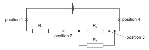
A student connects an ammeter first in position 1, then in position 2, 3 and 4 in turn.
