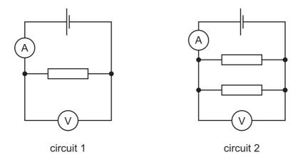
She then connects an identical resistor in parallel with the original resistor. She calls this circuit 2. She records current  $I_2$  and calculates the total resistance  $R_2$  of this circuit.
